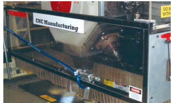
Fig. B. EXAIR's Cold Gun is mounted under the protective guard.
