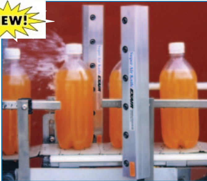
(2) Model 110012 12" Super Air Knives dry bottles prior to labeling.
