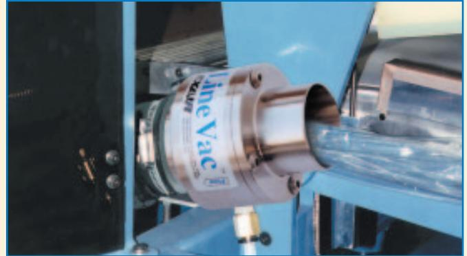
*A Model 6084 2" Line Vac conveys scrap plastic away from an "L" Sealer.*
