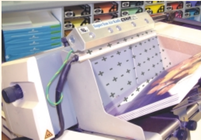
The Super Ion Air Knife eliminates jamming and assures crisp, clear printing of addresses on this ink jet machine.
