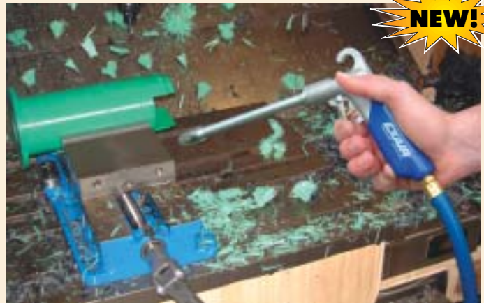
This Soft Grip Safety Air Gun with Super Air Nozzle blows a part and vise clean following a machining process.
