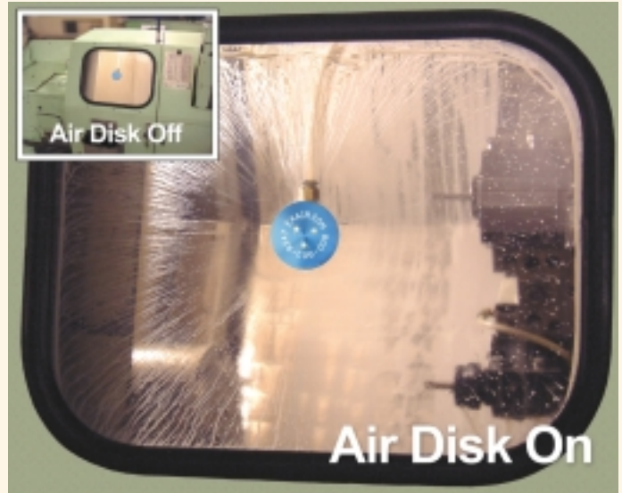
The Air Disk Window Blowoff creates a 360° airstream that blows out from the center of the window to keep it clear of coolant and chips.
