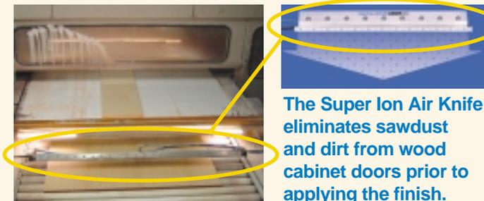
The Super Ion Air Knife eliminates sawdust and dirt from wood cabinet doors prior to applying the finish.
