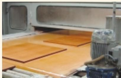
Airflow alone doesn't always do the job. Some products are charged with static electricity, attracting dust, lint and other contaminants. Our Super Ion Air Knife solves this problem. **An Ionizing Bar attached to the bottom of the Super Air Knife fills the forceful airstream with static eliminating ions to neutralize the charged surface, releasing the contaminants and blowing them away.**
