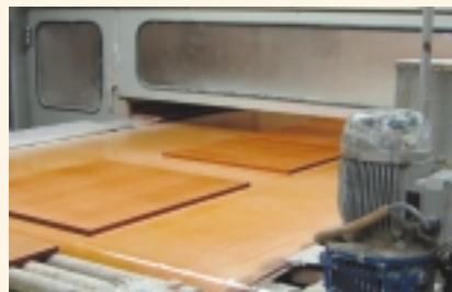
The Super Ion Air Knife eliminates sawdust and dirt from wood cabinet doors prior to applying the finish.
