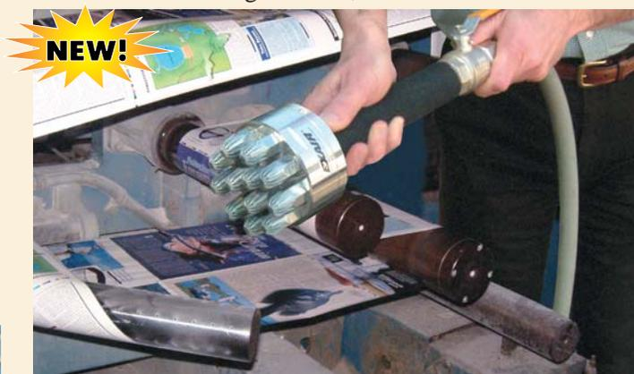
**The Model 1213-12 Super Blast Air Gun blows paper dust out of a web press with the airflow reaching deep into confined areas.**
