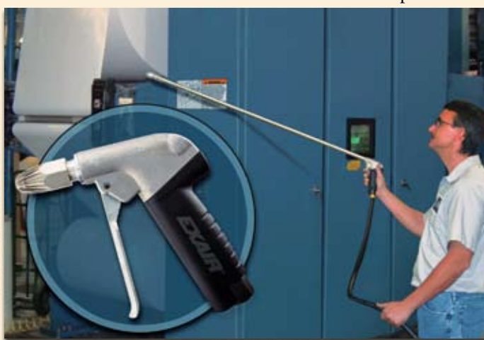
EXAIR's Heavy Duty Safety Air Gun blows paper dust off a web press.
