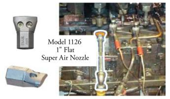
**SUMMARY:** The installation of an EXAIR engineered nozzle made this operation compliant with the OSHA directives for sound and dead-end pressure. A compressed air savings of 22.5 SCFM was achieved. Based on a one shift operation 250 days per year this amounted to 2,640,000 cubic feet of compressed air savings. (22 SCFM x 60min/hr x 8 hrs/shift x 250 days/year)
