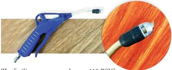
The facility operates at close to 110 PSIG with no regulators in place for their hand-held blow guns. Over an 8-hour period, their noise level testing averaged 90.7 dBA, measured at 12" away. In addition, the existing blow guns had failed safety features designed to reduce the outlet pressure below 30 PSIG, which also violated OSHA Standard 1910.242(b).
