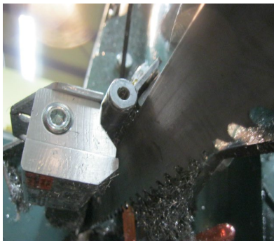
EXAIR Super Air Knives keep the chips away from the saw blade...
