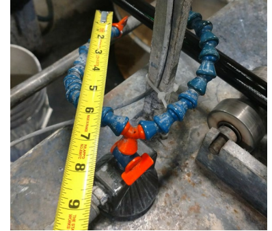
...but they're made for liquid. When used with air, they're inefficient and wasteful.
