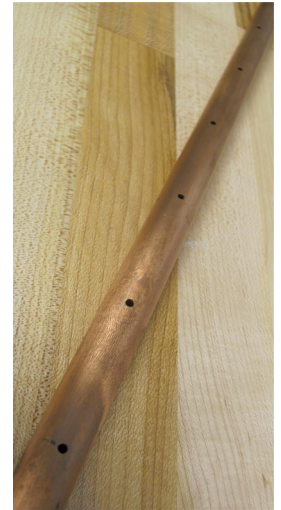
48" long copper pipe was tested in EXAIR's Efficiency Lab for performance. (23) 0.090" holes drilled along length.
