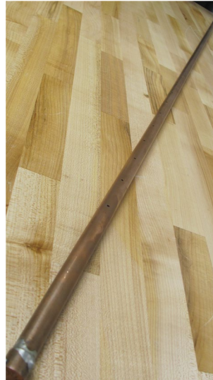
48" long copper pipe was tested in EXAIR's Efficiency Lab for performance. (23) 0.090" holes drilled along length.
