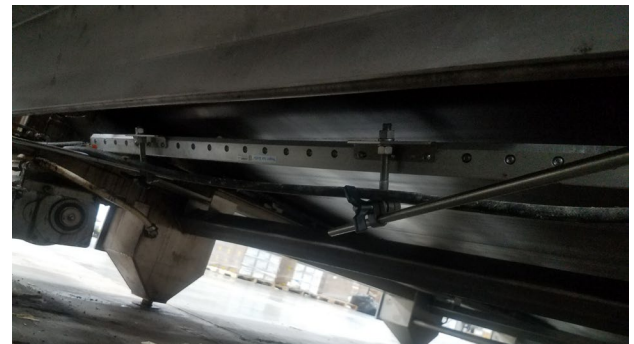
48" Aluminum Super Air Knife with 9060 Mounting System (above) keeps tortillas from flipping on the conveyor (right).
