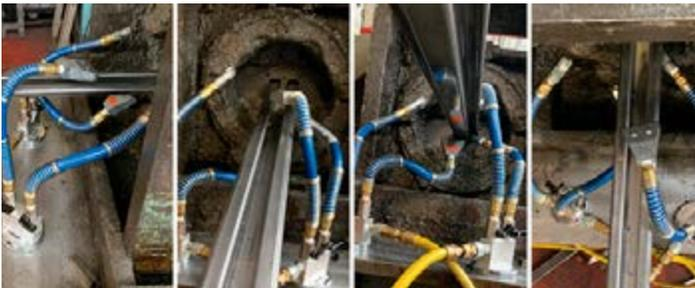
**AFTER EXAIR:** A Two Model 1100 Super Air Nozzles and two Model 1122 2" Flat Super Air Nozzles were purchased and installed (above) using Model 9043 Magnetic Bases and Model 9212 12" Stay Set Hoses. Coolant and debris were still effectively removed from the product. Compressed air consumption and noise levels dropped to 86.8 SCFM @100 PSIG, and 83.8 dBA, respectively.
