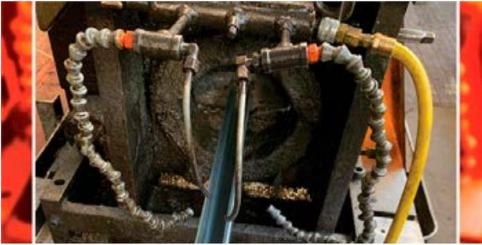
A producer of custom products needs to reduce compressed air consumption and noise levels associated with the use of coolant hose and copper tubing in a rollform blow off application.
