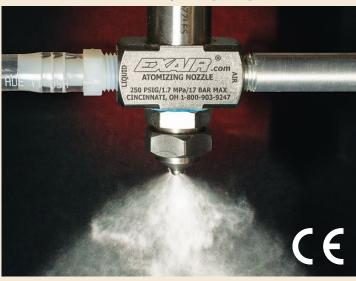
Siphon Fed Atomizing Spray Nozzles require no liquid pressure and can be used with gravity fed liquids or lift liquids from a siphon height as much as 36 inches (91cm). Siphon fed nozzles can be used on liquids up to 200 centipoise. The new No Drip Siphon Fed Atomizing Spray Nozzles work in the same way our standard atomizing nozzles do, but have the added benefit of positively stopping liquid flow when compressed air is shut off.
