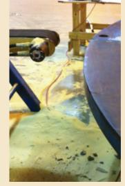
The picture to the right is an example of the buildup within the first hour of operation. It isn't long till the pile is knee deep, causing unstable footing for the operator. Towards the end of the shift, the saw has to be shut down to shovel up the accumulation and haul it away. At least an hour of production is lost per day.
