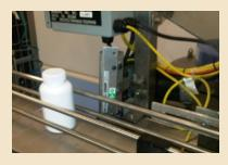
The Super Ion Air Knife Kits were installed to blow off both the bottle and the tamper proof sleeve. By installing **EXAIR Super Ion** Air Knife Kits, the
