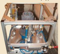
Air Knife Mounting Systems, and Model 9076 Air Knife Plumbing Kits.
