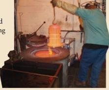
shop fans to cool the tooling piece from 1,725°F to less than 600°F. The engineer's intent was to provide a turntable system to rotate the part, while blowing it with a greater volume of air, to effect faster cooling. Their goal was to reach 600°F in 15 minutes.
