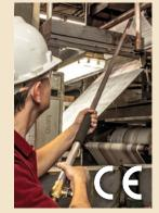
that force with the added benefit of being able to reach tight machinery spaces makes the Super Blast Safety Air Gun a great tool for wide area blowoff, cooling and drying. To learn more about these Super Blast Safety Air Guns, check them out online at <a href="https://www.exair.com/05/sbsagext.htm">www.exair.com/05/sbsagext.htm</a>.
