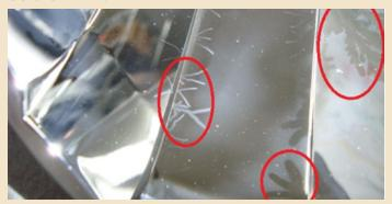
Injection molded parts were being direct metalized for use in automotive headlights. Parts were exiting the mold with a static charge and attracting dust prior to metalizing. The static charge and dust on the molded parts resulted in defects within the metalized coating in the form of spider webs and streaks in the coating. Any of these defects caused a rejection of parts and the manufacturer was experiencing close to 100% scrap rates.
